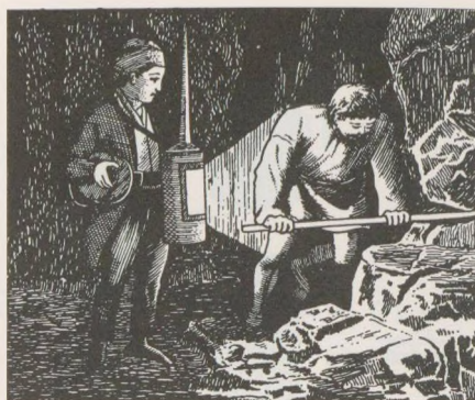
Fig. 7. Dr. William Clanny's blast lamp (second form). (From Hardwick and O'Shea, 18 p. 564.)
